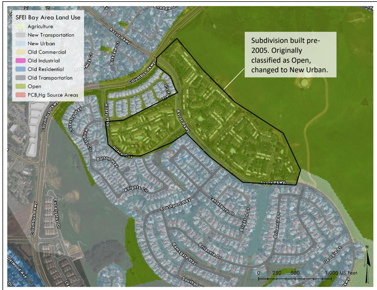
Figure 3.9. Example of a correction made in a Fairfield neighborhood to the land use layer used as input to the pollutant loading model.
